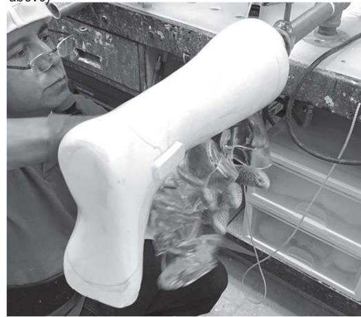
Fig. 2 Mount dummy to cast (see note above)
